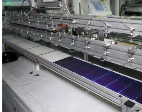
Solar panel welding machine
